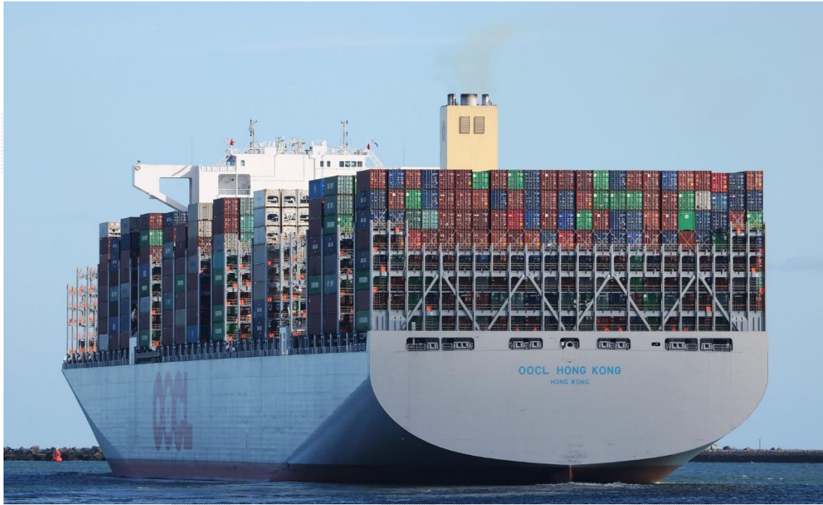
Figure 5 OOCL Hong Kong with a DWT (deadweight tonnage) of 191,317 metric tons, the OOCL Hong Kong has a cargo capacity of 21,413 TEU, making it the world's largest container ship
